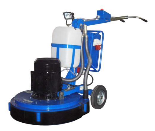
Planetary Grinding-Polishing Machine GPM-750 is the largest and the most productive machine in our product range. GPM-750 is used for high-productive and effective grinding of concrete, granite, mosaic, marble, wooden (including parquet) floors as well as for removal of old glue or paint coverings and final floor processing (polishing). The machine has EC Declaration of Conformity.
